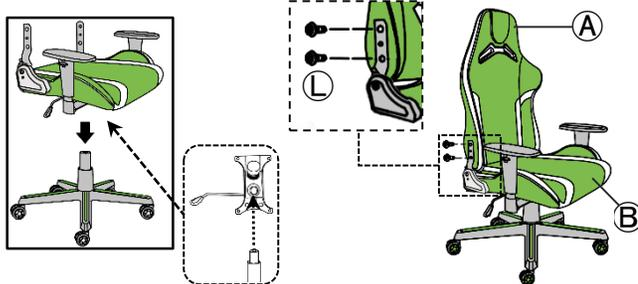
**STEP 5** Attach the covers (I-L) and (I-R) to the brackets on their respective sides of the seat (B) using screws (M) and cover the holes with (N) as shown.
