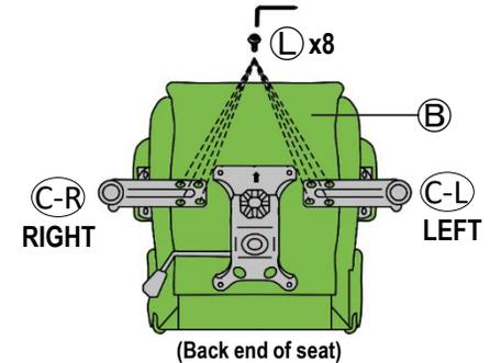
**STEP 4** Place the top parts over the base parts making sure the tip of the gas lift enters into the hole of the mechanism, then assemble the backrest (A) to the metal brackets on both sides of the seat (B) using screws (L) as shown.
