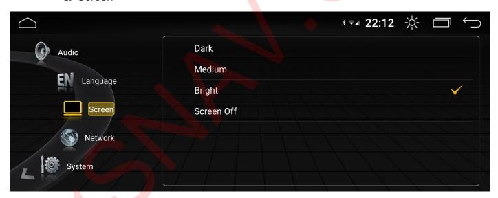
Regulates default screen brightness or turn the screen off until touched again. Even in the brightest setting, when headlight comes on, the backlight will be dimmer by 15%. To prevent this, activate the Brightness Override on the swipe down menu.
