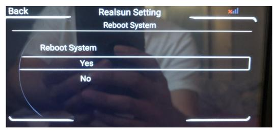
If your device is bricked, then disconnect the main connector, and plug the main connector back, this is to induce the bootloader to go to the download mode.
