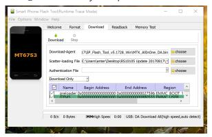
13. [Important]Go to 'Realsun Setting' app in the device again, and choose 'Restart the system'. Do not press 'Yes' yet. // If you bricked your device, this is the step that you disconnect the main connector.
