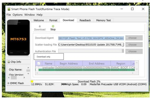
17. If thing are alright, you will see 'MediaTek PreLoader USB VCOM Port' is present and stay connected until the flash is complete. If the device didn't stay black out, and there is no progress in 'Flash tool', and the VCOM Port is not presented in the device manager, then your install the driver, again.
