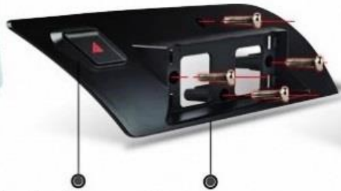
Replacement Hazard Flasher
