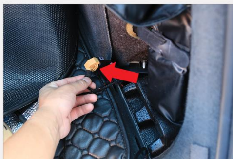
11. (Only for cars with the factory parkign sensors) Connect the supplied T-Bypas cable for the parking sensor information pickup.
