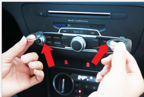
2. Using VAG Radio removal keys, remove Radio/MMI Headunit.
