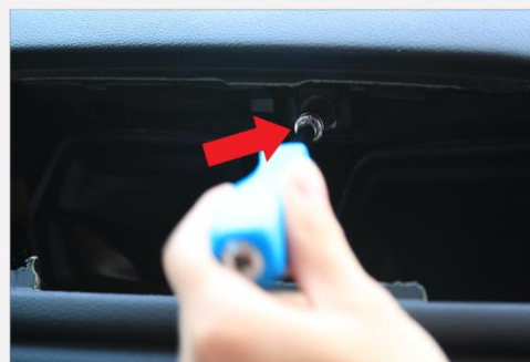
6. Unscrew the 8mm Hex screw holding the screen.
