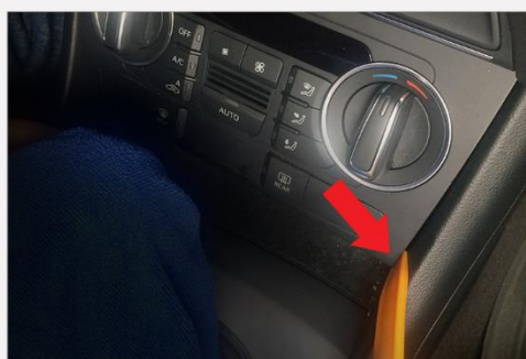
8. Pry out the climate control. Note: Pry the climate control from both side simultaneously.
