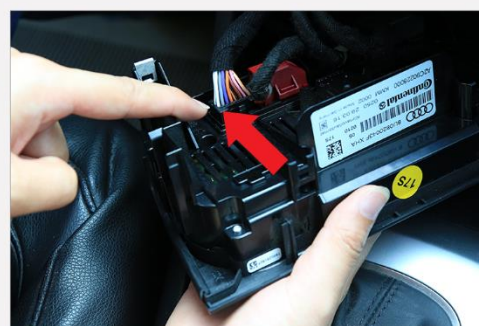
9. Unplug the climate control CAN BUS connector shown above.
