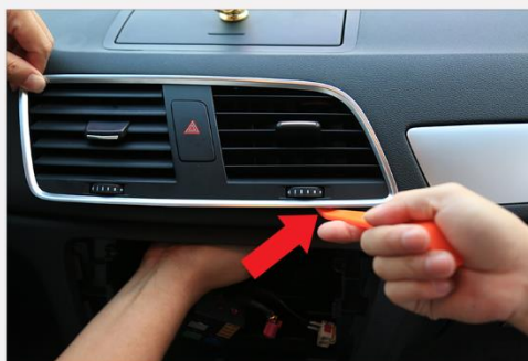
5. Remove the air vent using prying tool.
