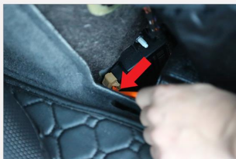
10.(Only for cars with the factory parkign sensors) Open the fuse panel cover in the trunk area located on rear right side of the vehicle and unplug the parking sensor module connector. Your car must be turned off.
