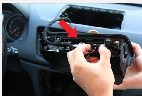
7. Pry up the original screen up with pry tool. Unplug all the plugs behind the original screen.
