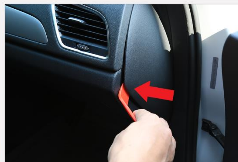
12. (Only for cars with the factory parkign sensors) Remove the passenger side fuse panel cover.
