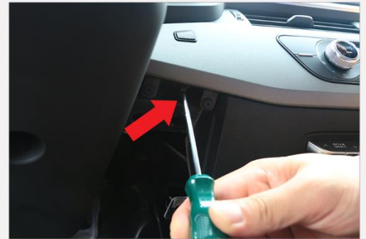
6. Remove the trim holding screw with T20 driver.
