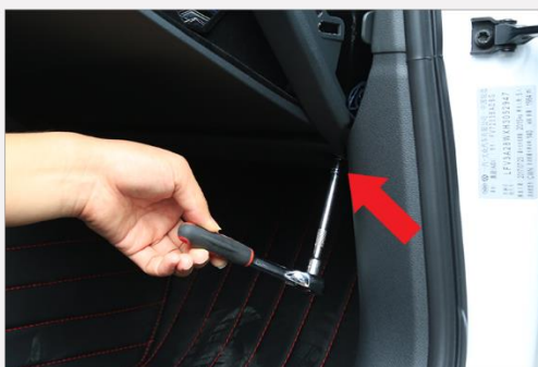
10. Remove 2 screws at the bottom of the glove box and unmount the glove box downward.
