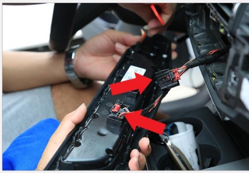
13. Unmount the climate control and unplug all the connectors.
