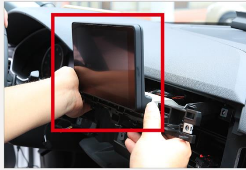
17. Remove the original screen by removing all the holding screws and disconnecting connectors.
