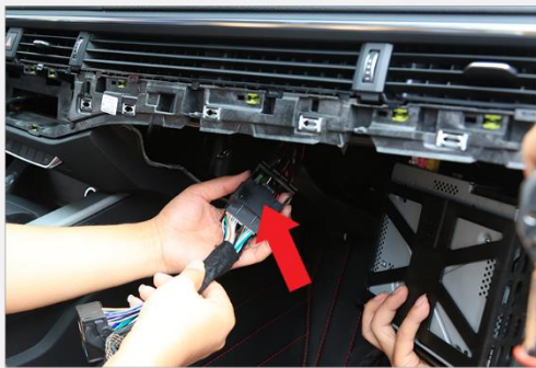
19. Install the provided main harness by routing the white main connector to the LCD screen area.
