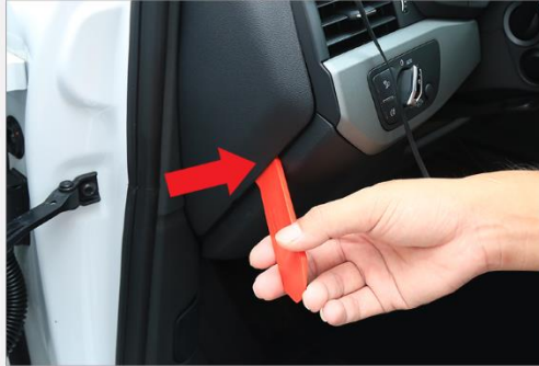
2. Using prying tool remove the driver side fuse panel cover
