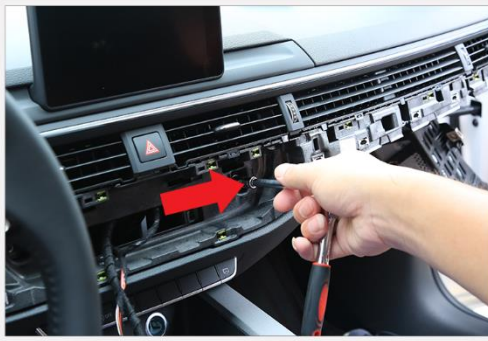
14. Unscrew 4 inside 8mm Hex screws
