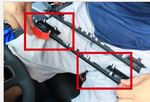
23. Transfer all the factory metal clips into new lower screen trim supplied with the kit and install it.
