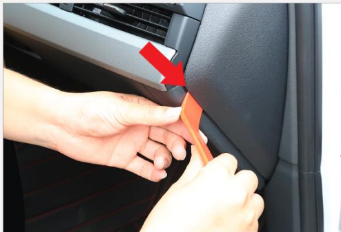
7. Using prying tool remove the passenger side fuse panel cover
