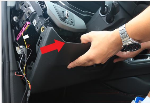
5. Remove the cover by pulling downward.
