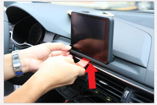
15. Remove the lower screen trim by prying from the bottom and pull the trim outward.
