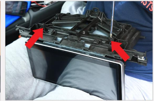
21. Install the new screen into the factory tray.
