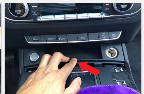
24. After the climate control trim installed properly, assemble back everything from installing the start button panel.
