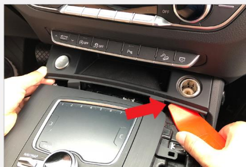
11. Remove the start button & cigarette socket assembly by prying for the bottom.
