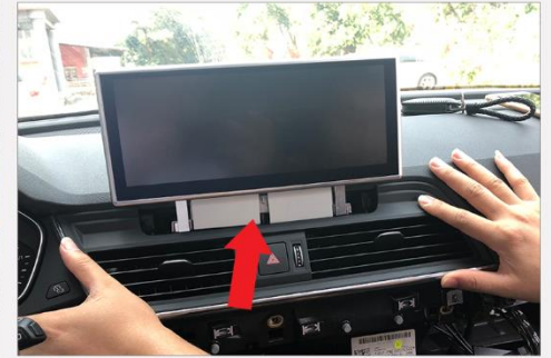
21. Place the new lower screen trim supplied (Reuse the factory metal clips for the trim).
