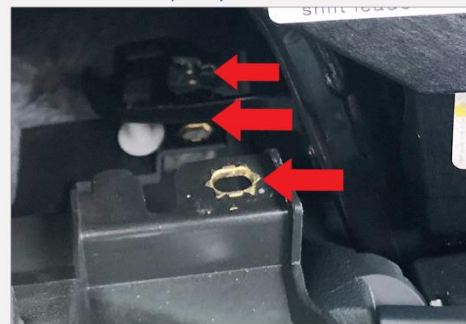
23. Reinstall the climate control trim, note: 1. Make sure the lower start button panel NOT installed before the climate control trim. 2. Make sure the left side of the climate control trim fits properly with the other loose trims such as lower instrument cluster cover and the driver knee board panel. Holes must align properly.
