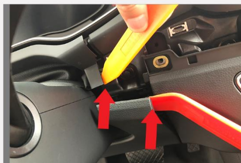
10. Pry the instrument cluster lower trim and the driver knee board panel slightly to remove the centre dash trim. IT IS NOT to remove them completely, but to have a bit of space to take out the center dash trim with climate control.
