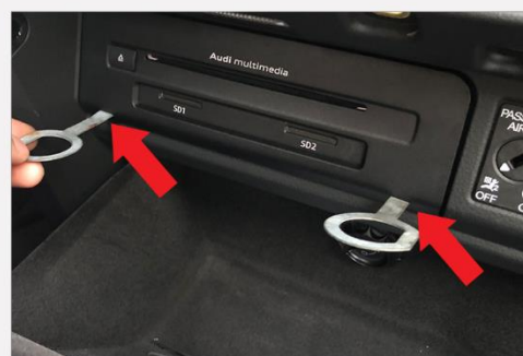
9. Remove MMI headunit using VAG Radio removal tool
