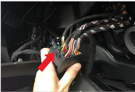
16. Install the provided main harness by routing the white main connector to the LCD screen area.
