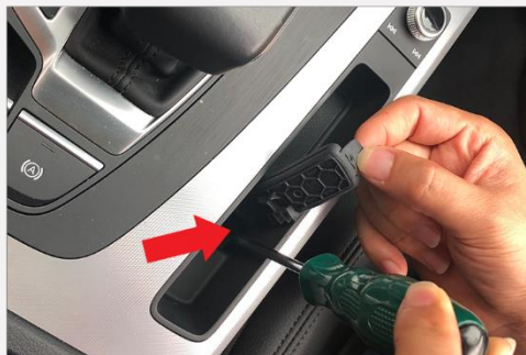
2. Unscrew the gear selector trim holding screw under the coin tray.
