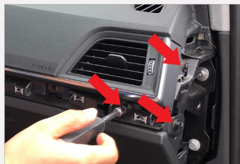
6. Remove all the 8mm Hex screws. Be careful that there may be additional screws not shown in the picture.
