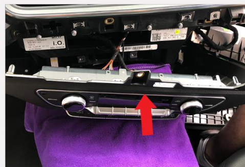
12. Unscrew the upper screw holding the centre dash climate control panel trim and carefully take out the trim.
