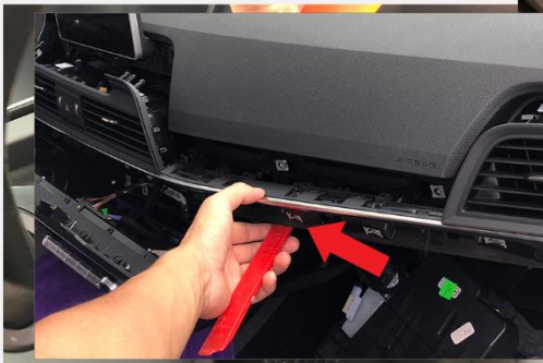
13. Pry out the center dash air vent frame assembly.
