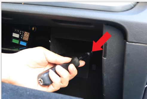
10. Remove the right side screw as well.
