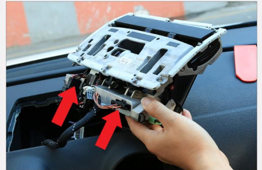
6. Remove the screen mechanism by removing LVDS connector and motor mechanism connector.
