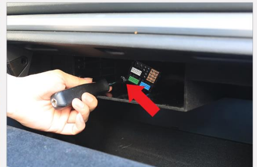
9. After unplugging every connector behind MMI unit, there is one 8mm hex screw to be removed. Unscrew it for further installation.
