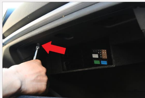
11. Unscrew every 8mm HEX screws that is holding the glove box compartment.
