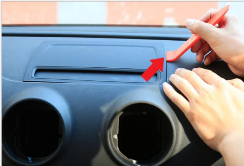
4. Pry up the screen cover trim and remove the trim.
