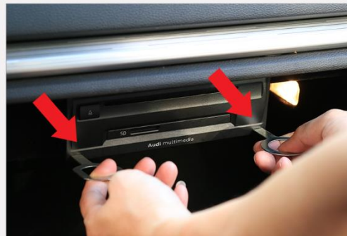
8. Remove the MMI headunit inside the glove box using VAG Radio removal keys.
