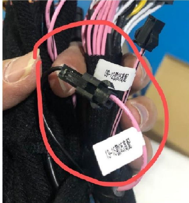
For 8.8" 3G MMI model there are single wire plugs tabbed with label saying 09-12 or 13-15, choose right one for your car model(Preface lift or facelift). This one is for automatic aux switching.
