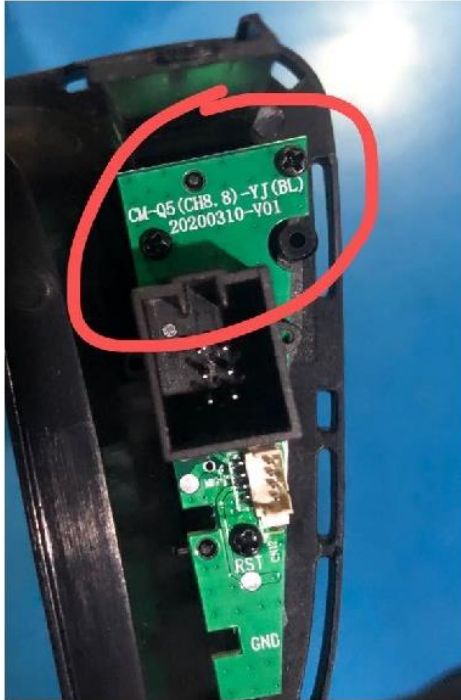
PCB with BL is for Pass. Airbag Off indicator equipped vehicle (e.g. the US)
