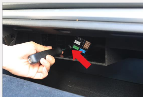
9. After unplugging every connector behind MMI unit, there is one 8mm hex screw to be removed. Unscrew it for further installation.
