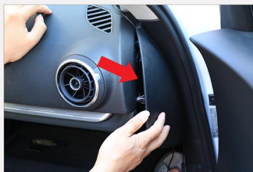
7. Remove the passenger side fuse panel cover.
