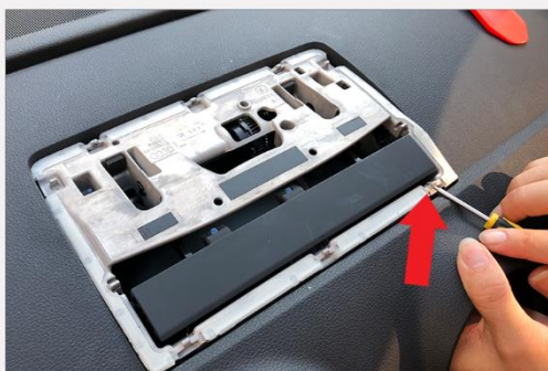
5. Using a hook, carefully lift up the screen mechanism assembly.
