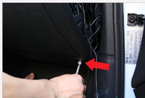
12. Remove the bottom screws for the glove box.
