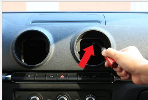
3. Unscrew the screen mechanism holding screws (one at each hole).
