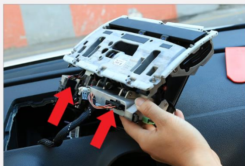
6. Remove the screen mechanism by removing LVDS connector and motor mechanism connector.
