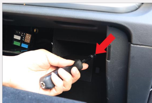
10. Remove the right side screw as well.
