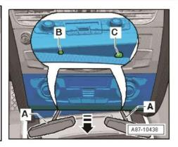
Using, VW radio removal tool, pull control unit 1 for infromation electronics –J794—1- out of mounting frame, and using -A- forklift tools, remove the climate control unit by pulling hook hole -B- and -C- together using the tools. Be careful when pulling out the climate unit as it is attached with four spring clips. Release and unplug necessary connectors at the behind of the control unit.
