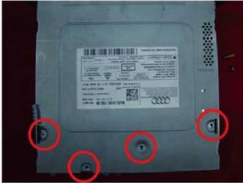
1. Remove The Navigation Host And Remove The Screws.
