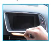
Remove the trim using a trim removing tool. Gently fry the gaps between the trim and the dash.
