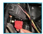
Disconnect the original CAN BUS wire (red connector) from interface inside the right corner of the glove box (Must turn off the car before disconnect)
