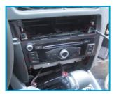
Remove the climate control and Using an 8mm Hex driver, unscrew four screws and pull
