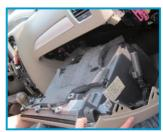
Pull the compartment down gently. Be careful for upper front side latches. Shake the compartment gently and latches the will be released
