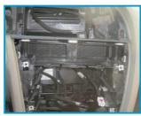
Disconnect and remove the radio. (If the gear knob interferes while removing, turn keys into ignition mode without pressing brake pedal and then press the pedal, switches gear knob to Drive, turn off the key)
