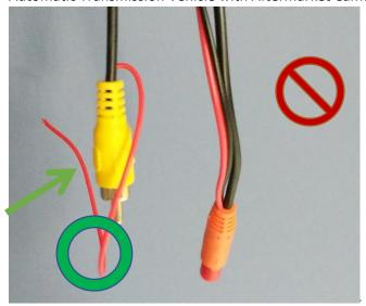
Do not use two wires (red and black) on the camera side. Connect the red wire near the yellow video side connector to the 'CCD PWR' bare wire of RSNAV S3, S4 main connector.
