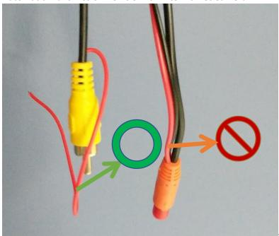
Do not use two wires (red and black) on the camera side. Connect the red wire near the yellow video side connector to the 'brown' bare wire of RSNAV main connector(white).
