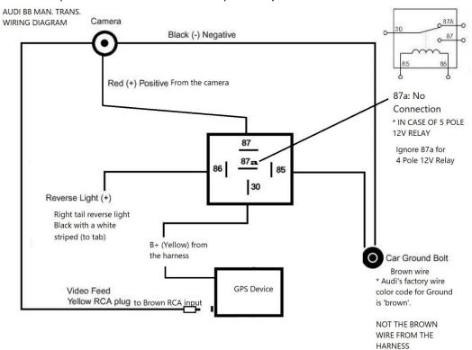
4. Manual Transmission Vehicle with Audi Original Camera, and Automatic reverse switching is not working
