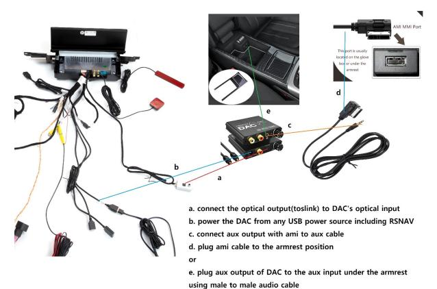
Following modification of T harness is required for the above optional sound routing.
