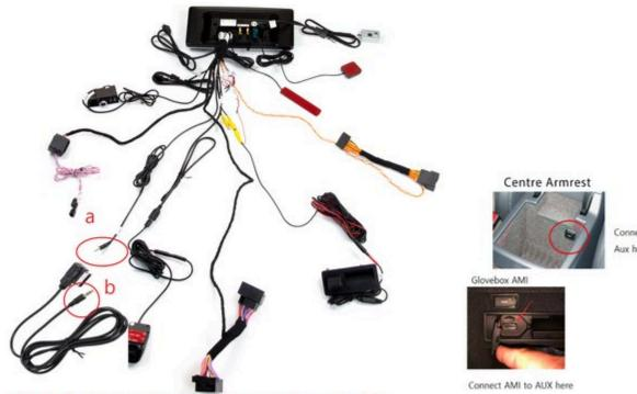
Only for concert/symphony radio a and b need to be connected. use double female 3.5mm audio aux adaptor. No coding for these radio.
