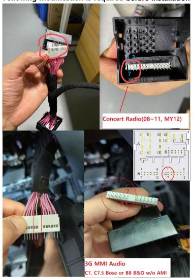
\*\*Note that block C pin 1,2,7 positions are different across radio type. You must cut the pins that is connected to white, black, and red line Not pink lines
