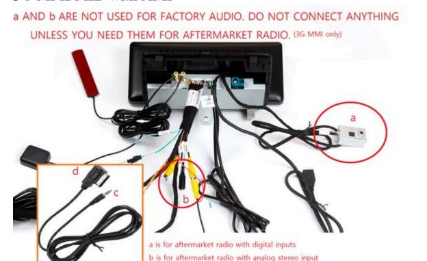
Do not connect AMI to AUX adaptor's audio plug to the the audio output of RSNAV S4.
