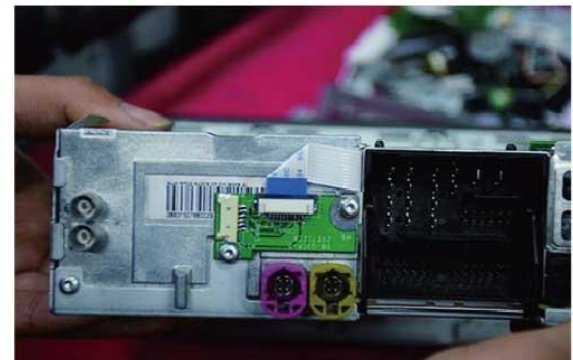
10. Install The External Adapter Plate , As Shown Above
