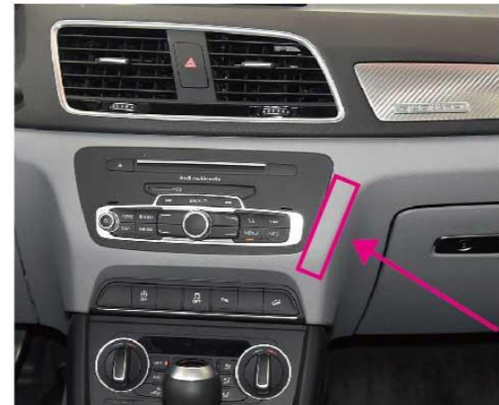
10. Install The External Adapter Plate , As Shown Above
