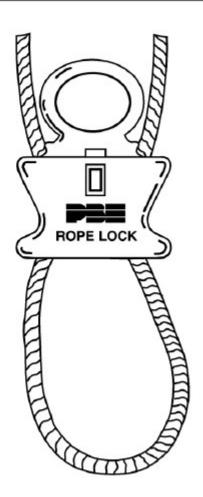
The P.B.E. ROPE LOCK is designed for #6 rope.
