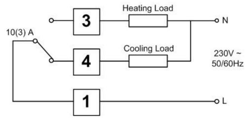
10(3)A (Resistive Load) or 3A (Inductive Load) No anticipator connection required
