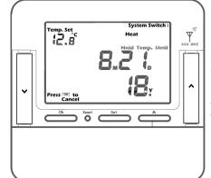
Hold Temp. Until is shown above the date on the display. Bottom right cycles between the set year and the room temperature.
