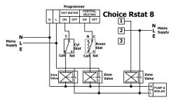
Choice RSTAT8 controlling a secondary heating zone on a pumped system with existing programmer and two spring return valves with auxiliary switches.
