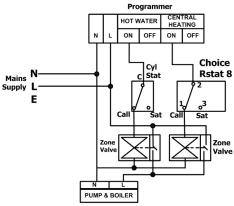
Choice RSTAT8 replacing a conventional room thermostat on a fully pumped system with an existing programmer and two spring return valves with auxiliary switches.
