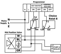
Choice RSTAT8 replacing a conventional room thermostat on a fully pumped system with an existing programmer and 3 port mid-position valve.
