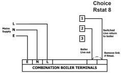
Choice RSTAT8 controlling a typical combination boiler installation - please refer to boiler manufacturers instruc-
