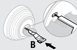
Insert the SmartKey tool (B) **fully and firmly** into the hole. You may feel the tool click inside the lock.
