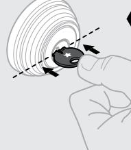
**Make sure new key (C) is FULLY inserted into lock.**
