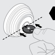
**⚠ Make sure new key is FULLY inserted into lock.**
