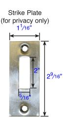
2" Screw-to-Screw <sup>1</sup>/<sub>16</sub>" Thick
