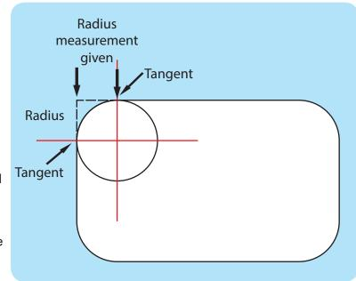
The diagram shows how to find the radius of a corner.
