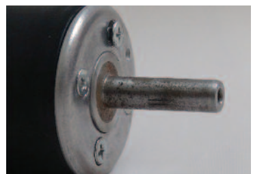
6. Putting screws back in place. Note diagonal tightening of screws.
