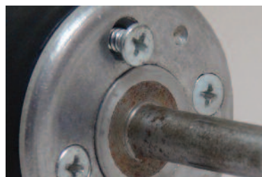
6. Putting screws back in place. Note diagonal tightening of screws.
