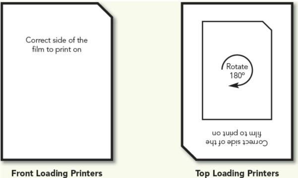
Feed film with corner notch to the right for 'face up' printers.
