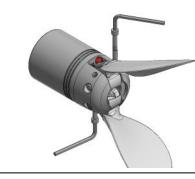
7 Release both anchor bolts approx. 1/8 turns counter clockwise (45 degrees). Check the function, i.e. work blades open and folded to insure ease of operation.
