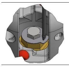
**2** Slide tab washer (5) on to shaft nut locking screw (6); screw in through hole in the shaft nut into end of shaft and tighten firmly; If using torque wrench tighten to about 15 Nm; (1,5 kpm, 10.8 ft-lb.)
