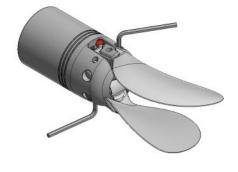
**8** Place the cover (10) as shown and click it into place. Finally work blades open and folded to insure ease of operation:
