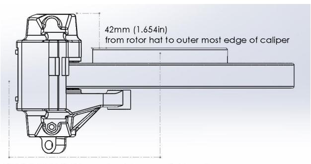
200MM(7.875 in) minimum wheel clearance inside radius
