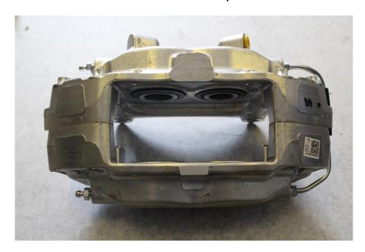
**With** your 10mm flare nut wrench, unbolt the crossover tube flare nuts. Then take your 11mm wrench and remove both bleeder screws.
