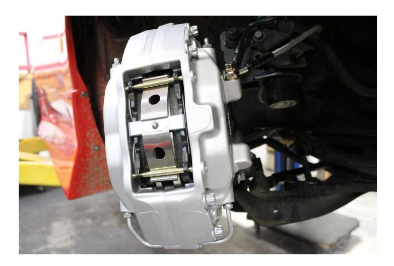
**Important note:** when bleeding fixed calipers with two bleeder screws. start with the inner most bleed screw. bleed until there are no air bubbles, then bleed the outer most bleed screw.
