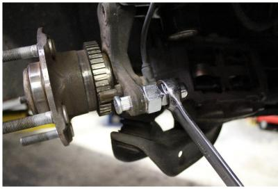
**Next,** we need to prepare for the caliper modifications. Mount the bracket to the knuckle. With your 18mm socket, tighten the nut to the bracket (thicker section towards the bottom, and angled towards the front) install the small spacer onto the top bolt.
