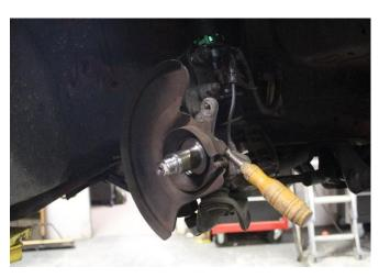
**Now** we need to file down two small edges on the lower caliper mounting ears so the bracket fits correctly.
