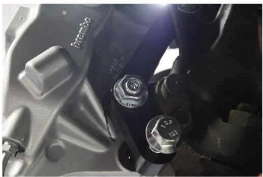
**Remove** the caliper and start shaving away material. periodically stopping to check that you have removed enough material.
