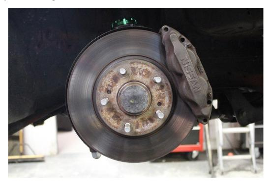
**Next,** with your 17mm ratchet loosen off and remove the stock brake caliper. Hang the caliper off to the side for now as to not spill brake fluid.
