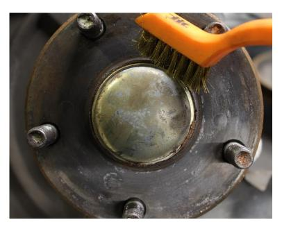
**Using** your 12mm wrench remove the backing plate/dust cover bolts. Once the bolts have been removed you can either press off the hub to remove as a whole, or cut a slit with an angle grinder and tear it off.
