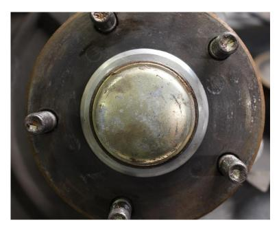
**Note:** if you're having troubles installing the ring make sure the hub is free of rust and debris, center the rotor overtop of the hub ring and firmly press.
