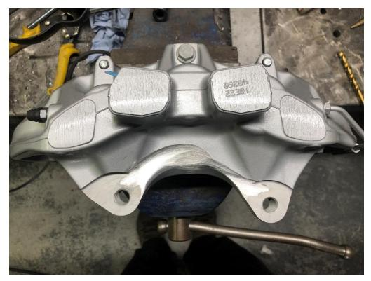
**make** sure to shave a bit extra off the flat section to allow more space for the bolt when mounted
