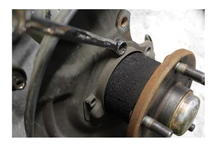
**Once** the backing plate has been removed, install the hub ring and rotor in preparation for the caliper.
