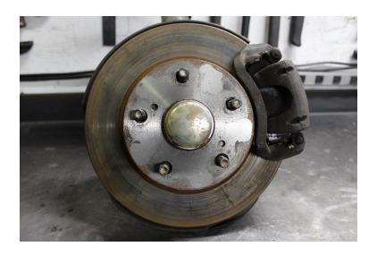
**Next,** with your 17mm ratchet loosen off and remove the stock brake caliper. pry between the rotor and caliper to get it free.
