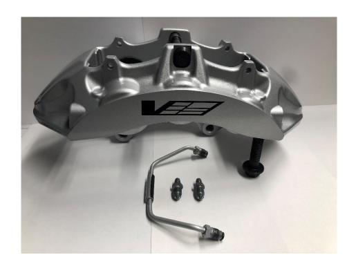
**Place** the bleed screws and crossover tube into their new orientation. The bleed screws should now be on the same side as the fluid inlet port as pictures below
