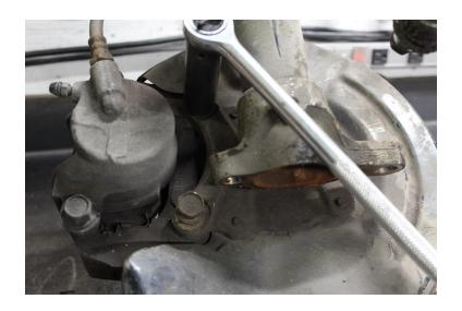
**Continue** by removing the stock rotor and brushing off any rust or debris with a wire brush, this step is important for when we install the supplied hub ring.
