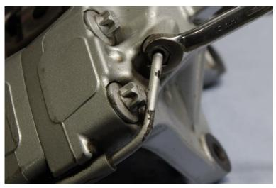
**Flip** the caliper over and remove the bleed screws with your 11mm wrench
