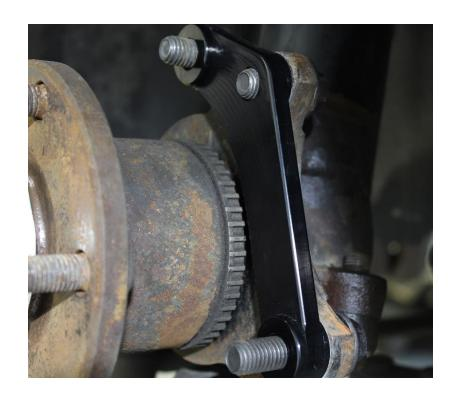
Note: 4 piston bracket pictured without rotor for reference
