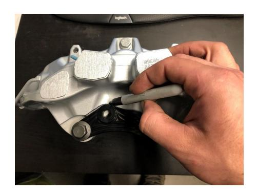
**With** your flap disk, begin removing material from the flat portion of the caliper up to the mark you made on the rib, occasionally stopping to check if the bracket sits flush on the mounting surface.
