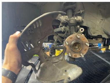
**Once** the backing plate has been removed, take your wire brush/wheel and clean both sides of the brake mounts, and the hub center.
