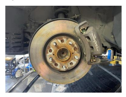
**Next,** with your 17mm wrench or ratchet, loosen off and remove the stock brake caliper. pry between the rotor and caliper to get it free. Hang the caliper off to the side for now as to not spill brake fluid.
