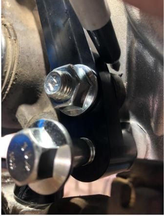
**Remove** the caliper and start shaving away material. periodically stopping to check that you have removed enough material.
