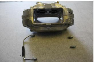
NOTE: Some calipers have asymmetrical crossover tubes and must be swapped with the ones from the other caliper.
