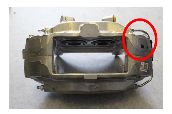
**Replace** the crossover tube and bleeder screws. Your caliper should now have the bleeders on the same side as the fluid inlet.
