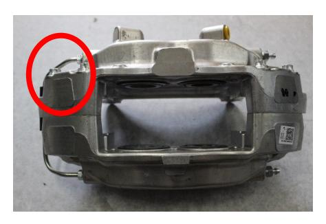
This below photo is for reference only, but take note of how much space there is between the bolt head and the crossover tube. This should stay consistent after swapping the lines and the bleeders.
