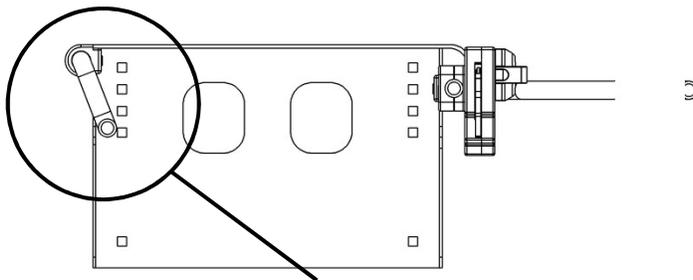
The bent steel rod installs at an angle as shown
