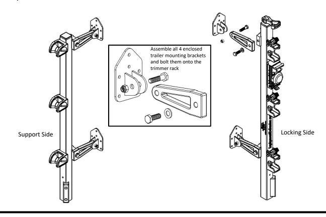
Step 2: Screw the brackets for the locking side onto the wall. Starting with the locking side, screw through the plywood and into the frame of the trailer. Note: check to make sure the screws aren't going to go through the outside wall of your trailer. Install as many screws as you can then remove the bracket from the rack and install the rest.
