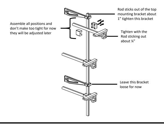
**Step 1: Install the engine support onto the locking side.** Install the top bolt first then slide the bottom bracket into position and install the bottom bolt. Tighten the bottom bracket so it can't
