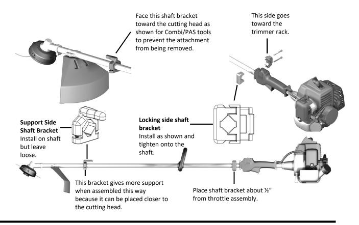
Step 2: Place the trimmer into the rack and adjust the support side shaft bracket
