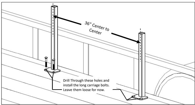
**Step 2: Install the "U" brackets.** Use a square to hold the post straight and mark the top rail of the trailer then hold the "U" bracket in place and mark the hole location for drilling. Drill 5/16" holes and install the "U" brackets tighten all of the bolts. **Note: The mounting posts must be parallel for your trimmer rack to function properly.**
