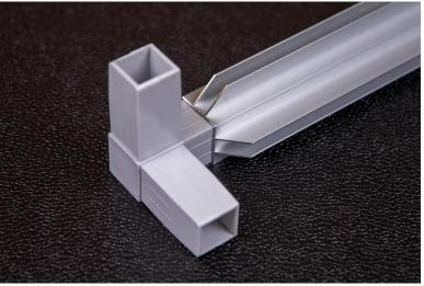
• Attach a 46" aluminum frame (Part A) and 46" bottom door frame (Part E) to one of the side frames with the corners attached. Make sure that the double door track is facing up and the inside channels all align. The frame and channels should now be in the shape of a U.
