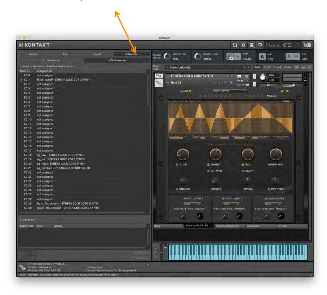
In this case the Assignable Table is set on MIDI\_CC 1 which is modulating the Filter Cut-Off.
