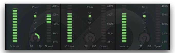
Starting from the left we have a standard volume fader, then we get on to the more interesting speed and pitch controls.
