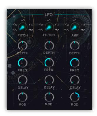
Epica has 3 x LFO's and each LFO has 5 Waveforms: Sine, Triangle, Saw, Square and Random.
