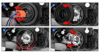
Insert the LED car light into the lampshade of the vehicle and fix it with the bulb spring
