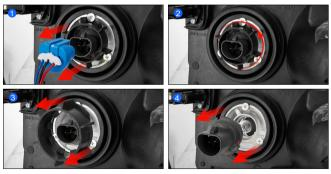
Insert the LED bulb into the vehicle housing, turn it clockwise and lock it in place.
