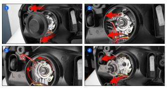
2. Holding the bulb by the heat sink, twist the locking ring counterclockwise until it unlocks, and then remove it.
