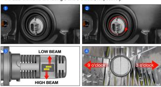
4. Connect the LED bulb connector with the original vehicle connector, then reinstall the rubber cover (if present).
