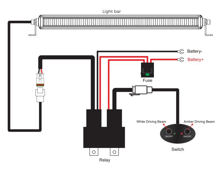
(Tips: 50" light bar use 12 AWG one-output wiring harness, other sizes use 14 AWG one)
