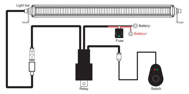
(Tips: 50" light bar use 10 AWG one-output wiring harness, other sizes use 14 AWG one)
