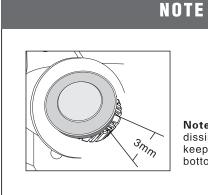
Note: To make heat dissipation better,please keep 3mm distance from the bottom of fan to dustcover.
