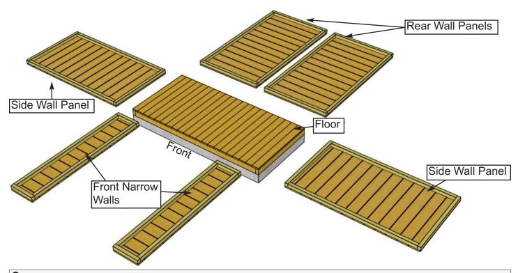
**3.** With Wall Plates properly attached, orientate completed Walls around the Floor. Be sure to leave room to work. **Front Narrow Walls** will be required in this section.
