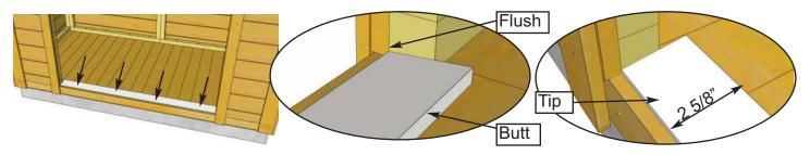
**57.** Locate **Door Threshold** and position on Floor at the opening. Align tip of the bevel flush with the outside of Bottom Wall Plate. Attach with **4 - 1 1/4" Brown Screws.**
