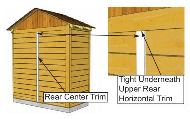
**51.** Locate **Rear Center Trim.** Align tight against Upper Rear Horizontal Trim and attach with **6 - 1 1/2**" **Finishing Nails.**
