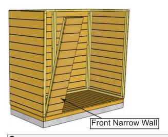
**9.** Locate **Front Narrow Walls** and position Wall framing flush with Side Wall framing in corner. **Important: Make sure Narrow Wall is positioned right side up.**
