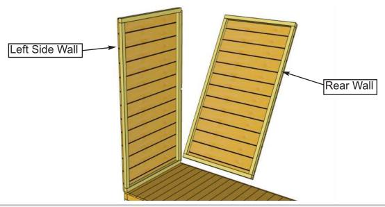
**5.** With your helper holding the Side Wall Panel, position a **Rear Wall Panel** in rear corner. **Important: Align Wall Framing Flush with Floor Framing.**
