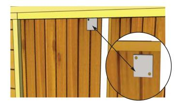
**65.** Install the **Plywood Spacer** to interior Door frame approximately 1 1/2" from top of Door frame and 1" from edge, as pictured. Use **2 - 1** 1/4" **Brown Screws** to secure. Plywood Spacer should fit flush underneath Interior Door Header when Door is closed.
