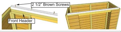
**16.** Locate **Front Top Plate** and place on top of Front Header. With Front Top Plate positioned evenly and flush against Front Header, secure using **6 - 2 1/2" Brown Screws** screwing down from the top of Front Top Plate down into Front Header.
