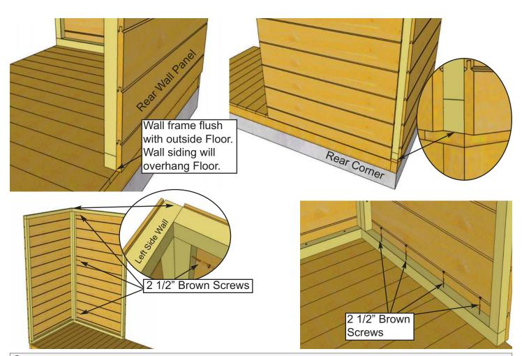
**6.** When Side and Rear Walls are aligned in corner correctly, Wall framings will be flush. Attach Wall framings together with **3 - 2 1/2" Brown Screws**. Secure Bottom Wall Plate to Floor with **4 - 2 1/2" Brown Screws**.
