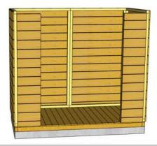
**11.** Align and attach the second **Front Narrow Wall Panel** as per **Step 10**.
