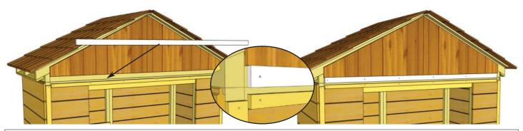
**44.** Locate **Front Top Plate Filler Strip.** Position Front Top Plate Filler Strip onto Front Top Plate. Evenly space from side to side. Secure with **6 - 1 1/2**" **Finishing Nails** into Front Top Plate.
