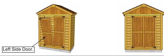
**61.** Position Left Side Door (with Flange) as per **Step 60**. Once again, use only **1 - 2" Black Headed Screw** per Hinge initially to secure door to Vertical Door Frame Trim.
