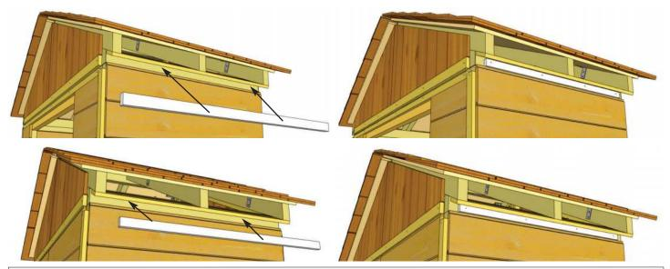
**46.** Locate an **Upper Horizontal Side Wall Filler Trim.** Position on Side Wall Top Plate. Evenly space from side to side. Secure with **4 - 1 1/2" Finishing Nails** into Side Wall Top Plate. Complete opposite side with same positioning and attachment.
