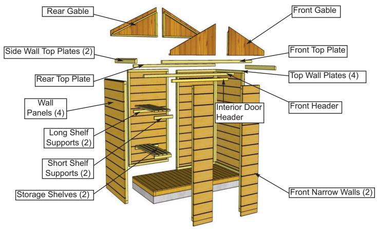
Due to packaging constraints, top wall plates must be attached prior to erecting walls.
