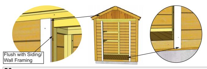
**56.** Locate 2 **Vertical Door Frame Trims.** Position on Front Narrow Wall flush with Wall siding/ framing and underneath Front Header Filler Strip. Attach with **6 - 1 1/2**" **Finishing Nails.**
