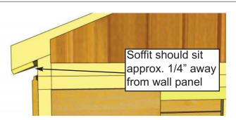
**30.** When Rafter section is correctly positioned, outside rafters will sit equally on Gable framing and soffit will sit approximately 1/4" away from wall panels.
