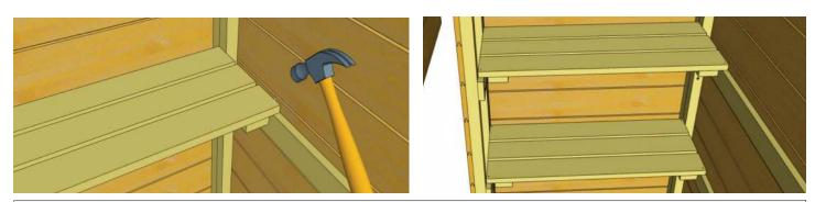
**23.** Place **Storage Shelf** on top of supports and secure with **4 - 1 1/2**" **Finishing Nails**. Complete 2nd Shelf (if desired) as per **Steps 22 & 23**.
