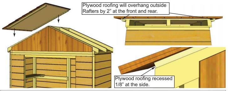
**36.** Lift up first **Cedar Shingle Roof Panel** and place on Rafters. At the front and rear, plywood roofing should overhang Rafters by 2" and recessed 1/8" back from Rafters at the side.
