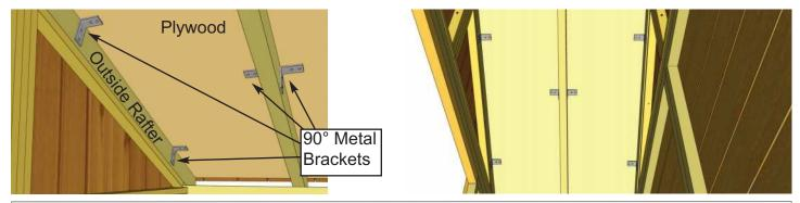
**37.** Inside the shed, position 6 - 90° Metal Brackets onto the Roof plywood and Rafters and secure with 4 - 3/4" Silver Screws each Bracket. For each Roof Panel, 4 - 90° Metal Brackets will be used for the outside Rafters and 2 - 90° Metal Brackets will be used to secure the middle Rafter.
