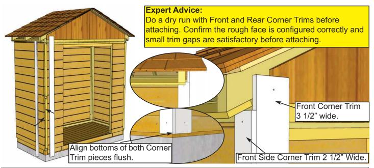
**47.** Locate a **Front Wide Corner Trim** and **Side Corner Trim**. Starting in one corner, position both Trims up underneath Cedar Roof and Soffit. Align Front Wide Corner Trim with bottom of Side Corner Trim. Side Corner Trim will cap Front Wide Corner Trim. When correctly aligned, attach each piece with **6 - 1 1/2**" **Finishing Nails**.
