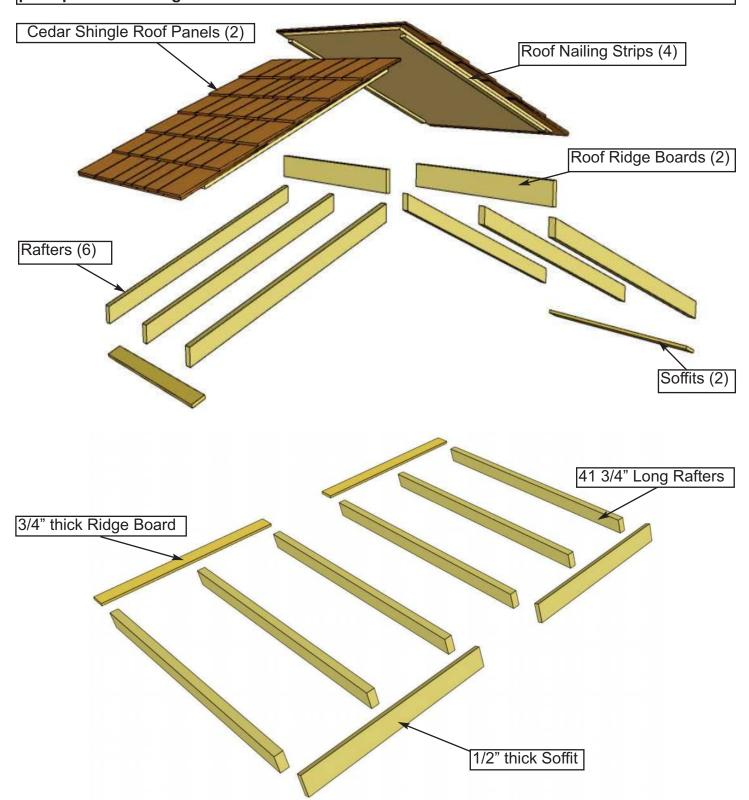
**24.** Locate 6 **Rafters**, 2 **Ridge Boards**, and 2 **Soffits**. Evenly space out Rafters and lay out as illustrated, on a flat level surface.
