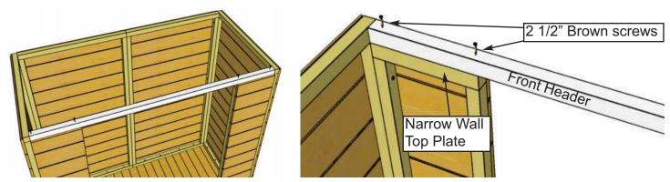
**13.** With Front Header positioned evenly on Narrow Wall top plates and flush against Side Wall top framing, secure using **4 - 2 1/2" Brown Screws** screwing down from the top of Front Header down into the upper Narrow Wall plates. Have your helper push side walls against end of Front Header to achieve tight fit if possible.
