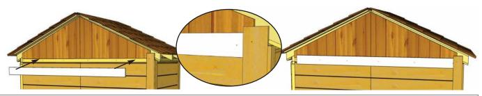
**50.** Locate **Upper Rear Horizontal Trim** and align tight against Rear Wide Corner Trim. Attach to Rear Top Plate Filler Strip with **6 - 1 1/2**" **Finishing Nails**.
