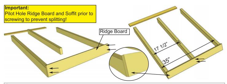
**25.** Starting with first Rafter section, attach Ridge Board to ends of both outside rafters with **2 - 2" Brown Screws** per end. Drill 1/8" pilot holes in Ridge Board to prevent splitting. Measure and position interior Rafter as illustrated. When positioned correctly, attach Ridge Board to remaining Rafter with **2 - 2" Brown Screws**.
