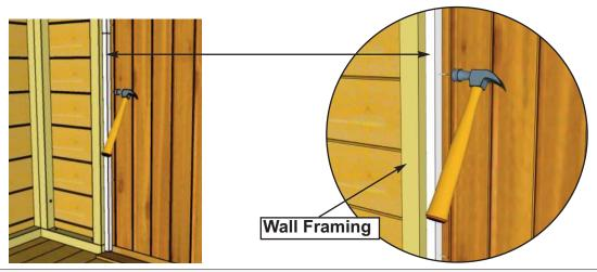
**68.** Attach **Interior Vertical Door Stops** to inside Wall framing with **4 - 1 1/2**" **Finishing Nails** per piece. To align correctly, close Door to make sure Stops are close to the Door but don't interfere with their closing. Attach bottom piece first with hammer.
