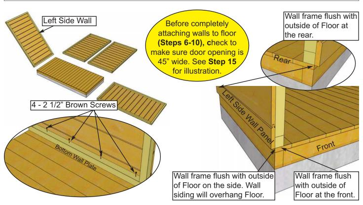
**4.** Starting with **Left Side Wall**, lift up and position so framing is flush with Floor at both front and rear of shed. Make sure Wall frame is flush with outside of Floor on the side. When Wall is positioned correctly, secure Bottom Wall Plate to Floor with **4 - 2 1/2" Brown Screws.**
