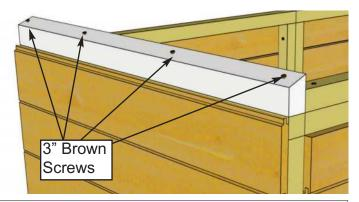
**17.** Locate and position first **Side Wall Top Plate** on Side Wall frame so they are flush. Side Wall Top Plates are angle cut down the length. Attach Side Wall Top Plate to Side Wall framing with **4 - 3" Brown Screws.**
