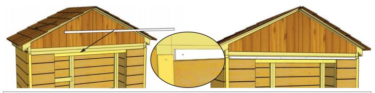
**43.** Locate **Front Header Filler Strip.** Position Front Header Filler Strip onto Front Header. Evenly space from side to side. Secure with **6 - 1 1/2**" **Finishing Nails** into Front Header.
