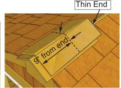
**71.** Place first **Roof Ridge Cap** on Roof peak overhanging shingles by approximately 1". Attach with **2 - 1 1/2" Shingle Nails** 9" from end. Place second **Ridge Cap** 1" back from first Ridge Cap. Attach with **2 - 1 1/2" Shingle Nails** 9" from end. Alternate each Ridge Cap seam as you proceed.
