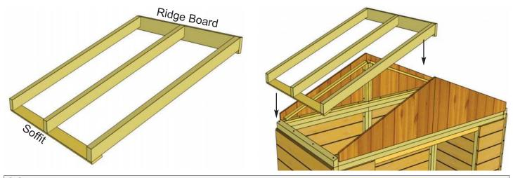
**28.** Flip Rafter section over so Soffit is facing down. Starting with one side, lift completed Rafter Section up and place on Gable framing.
