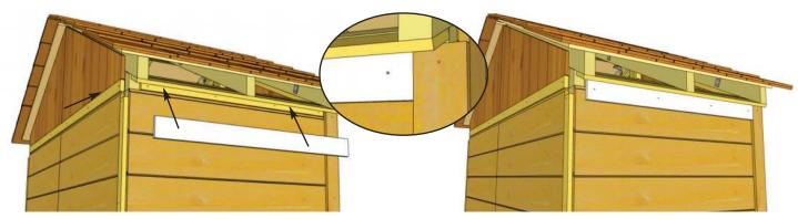
**48.** Locate **Upper Horizontal Side Wall Trim** and align tight against Front Side Corner Trim. Attach to Upper Horizontal Side Wall Filler Trim with **4 - 1 1/2**" **Finishing Nails.**
