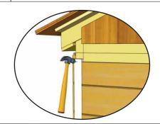
**41.** Locate 4 **Front Filler Trims.** Filler trim will be covered by Corner Trim in **Step 47**. Attach in each front corner with **3 - 1 1/2**" **Finishing Nails** per piece.
