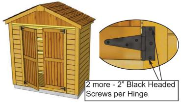
**62.** With both Doors partially attached, check to see Doors open and close correctly. Make any necessary adjustments and when satisfied, completely secure Hinges to Vertical Door Frame Trim with **two** more **2" Black Headed Screws** per Hinge. Drill pilot holes to prevent wood from splitting.
