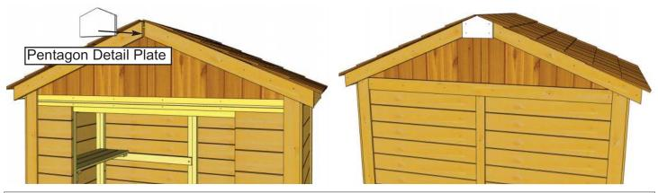
**55.** Attach **Pentagon Detail Plates** where Front and Rear Fascia Trims meet at the peak. Secure with **4 - 1 1/2**" **Finishing Nails** per piece.
