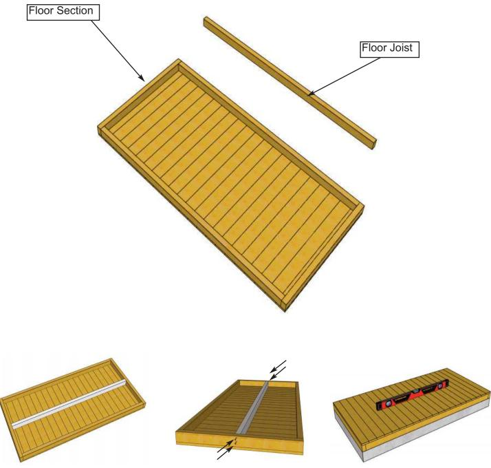
1. Locate Floor Joist and position at center of Floor Section and flush with framing as illustrated above. Attach with 2 - 2 1/2" Brown Screws per end. Flip over and lay Floor Section on a level foundation only. Patio Stones or a Concrete Slab both make excellent foundations. (See Page 3 for more information on foundations). Use a level to confirm and shim Floor Joist as required.
