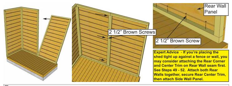
7. Position second Rear Wall Panel on Floor as per Step 6. Attach Wall frames together at top, middle and bottom with 3 - 2 1/2" Brown Screws. Secure Bottom Wall Plate to floor with 4 - 2 1/2" Brown Screws. Important: Confirm Siding on Rear Wall Panels are aligned.
