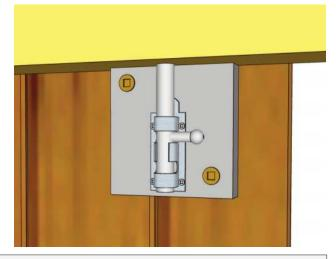
**67.** Open Door and drill out marked Silver Barrel Bolt impression with a 3/8" Drill Bit. Close Door, slide Interior Silver Barrel Bolt in drilled hole to confirm fit.
