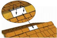
**72.** Place third **Ridge Cap** 8" back from second (enough to cover shingle nails). Attach third Ridge Cap as per **Step 71**. Continue to position and attach Ridge Caps until half the Roof is complete. From opposite side, position and attach Ridge Caps as described above. One Ridge Cap is cut shorter to fit in the center of the Roof. Attach **Center Ridge Cap** with **4 - 1 1/2**" **Shingle Nails**.
