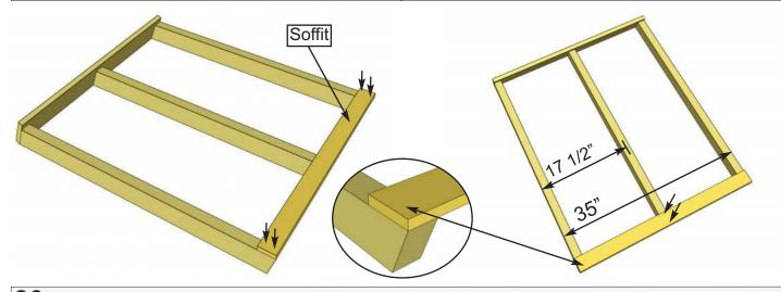
**26.** Attach end of Soffit Board flush to ends of outside Rafters with **2 - 1 1/4**" **Brown Screws** per rafter end. Drill 1/8" pilot holes in Soffit ends to prevent splitting. Measure and position interior Rafter as illustrated. When positioned correctly, attach Soffit to remaining Rafter with **2 - 1 1/4**" **Brown Screws.**
