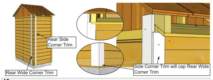
**49.** Locate a **Side Corner Trim** and **Rear Wide Corner Trim** and position both Trims up underneath Cedar Roof and Soffit. Align Rear Wide Corner Trim with bottom of Side Corner Trim. Side Corner Trim will cap Rear Wide Corner Trim. When correctly aligned, attach each piece with **6 - 1 1/2" Finishing Nails.**
