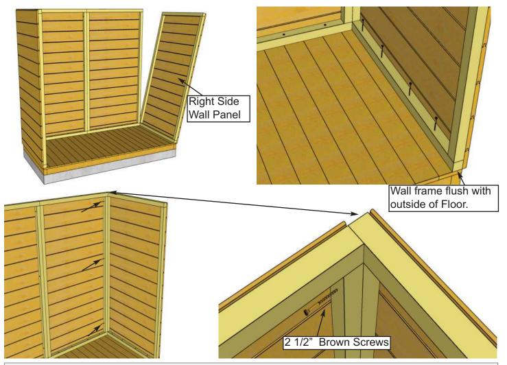
8. In the corner, align and attach Right Side Wall framing to Rear Wall framing with 3 - 2 1/2" Brown Screws as per Step 6. Secure Bottom Wall Plate of Side Wall to Floor with 4 - 2 1/2" Brown Screws.
