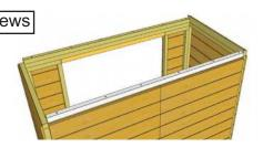
**18.** Locate **Rear Top Plate** and place on top of Rear Walls. With Rear Top Plate positioned evenly and flush against Rear Wall framing, secure using **6 - 2 1/2" Brown Screws** screwing down from the top of Rear Top Plate down into the Rear Wall top plates.
