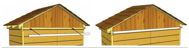
**45.** Locate **Rear Top Plate Filler Strip.** Position between Rear Walls and Rear Gable. Evenly space from side to side. Secure with **6 - 1 1/2**" **Finishing Nails** into Rear Top Plate.
