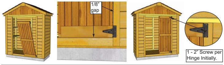
**60.** Starting with Right Door first, lift and position Door in opening. Leave a 1/8" gap on right side and 1/8" gap on the bottom. Use a **Cedar Shingle Shim** to shim the Door at bottom to help position door evenly. When Door is aligned correctly, screw Hinge into Vertical Door Frame Trim with **1 - 2**" **Black Headed Screw.** Use only 1 screw initially per Hinge until both Door alignments are confirmed. Drill pilot holes to prevent wood from splitting.
