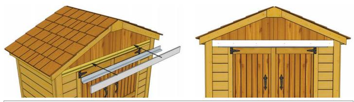
**70.** Locate **Front Horizontal Trim** and **Metal Drip Edge**. Position Metal Drip Edge behind Door Trim. Evenly space from side to side. While holding down both Metal Drip Edge and Front Horizontal Trim, secure with **6 - 1 1/2**" **Finishing Nails** into Front Header Filler Strip.
