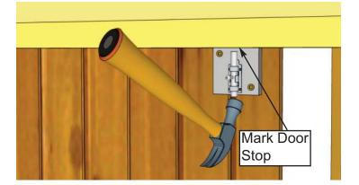
**66.** Position the **Interior Silver Barrel Bolt** on the Plywood Spacer and attach with **4 - 3/4" Silver Screws.** Tap Silver Barrel Bolt with hammer on underside of Interior Door Header to mark location.
