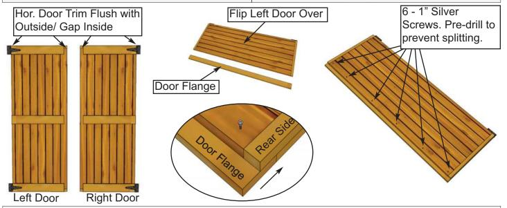
**59.** Flip Left Door over to attach **Door Flange.** Position Door Flange tight against horizontal trim and even with trim on top and bottom. If out slightly, make sure top horizontal trim and Flange are even. Pre-drill with 1/8" bit to prevent wood from splitting. Attach with 6 - 1" **Silver Screws.**
