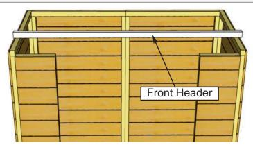
**12.** Locate **Front Header** and place on top of Front Narrow Wall framings.
