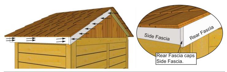
**53.** Position Rear Fascia (angle cut on ends) and Side Fascia (square cut ends) in corner. Line Fascia up so Rear Fascia caps Side Fascia. Attach Rear Fascia to Nailing Strip with 6 - 1 1/2" Finishing Nails and Side Fascia to ends of Rafters with 6 - 1 1/2" Finishing Nails. Gap where Fascia boards come together at peak will be covered in **Step 55.** Do a dry run using Side Fascia to help you correctly position before attaching.
