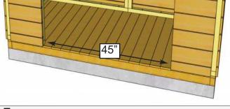
**15.** When all Walls are attached together, check door width at top and bottom. Door width should be 45" wide. If required, loosen Narrow and Side Wall plate screws, adjust door width and re-secure. There can be an 1/8" tolerance in the width but top and bottom width should be the same.
