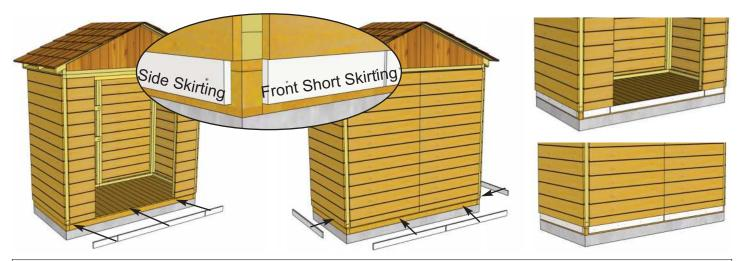
**40.** Locate **Lower Front Skirting (2 Short and 1 Long).** Skirting will hide floor framing. Gaps will be covered by Wide Trim pieces later. Attach 2 Lower Short Front Skirting pieces with **2 - 1 1/2" Finishing Nails** per piece. Attach Lower Front Long Skirting with **4 - 1 1/2" Finishing Nails.** Locate **Lower Side and Rear Skirting** and attach with **4 - 1 1/2" Finishing Nails** per piece.
