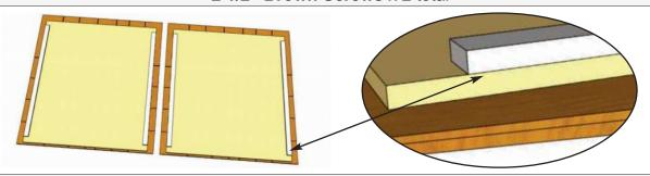
**35.** Carefully flip **Cedar Shingle Roof Panels** over so plywood is facing up. Attach **Roof Nailing Strips** onto outside of each panel flush with plywood. Attach with **3 - 1 1/4" Brown Screws** evenly spaced. Nailing Strips provide for a greater nailing surface later when you attach Front/Rear Fascia Trim.
