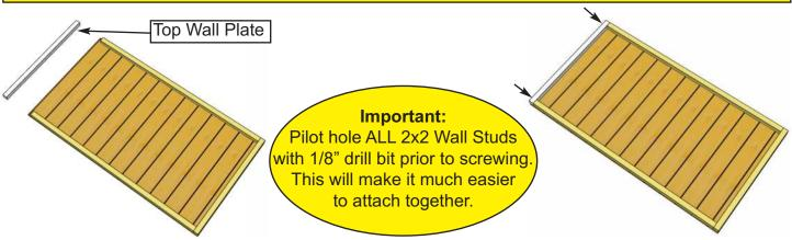
**2.** For each **Rear and Side Wall Panel**, carefully lay Panel face down. Position and attach a **Top Wall Plate** to top of wall studs of each Wall Panel with **2 - 2 1/2" Brown Screws**. Position so Plates are flush with framing.
