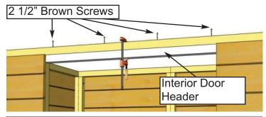
**14.** Position Interior Door Header underneath and flush with Front Header. Attach with 4 - 2 1/2" Brown Screws. Screw down from the Front Header into Interior Door Header. Use Clamp to hold Interior Door Header.
