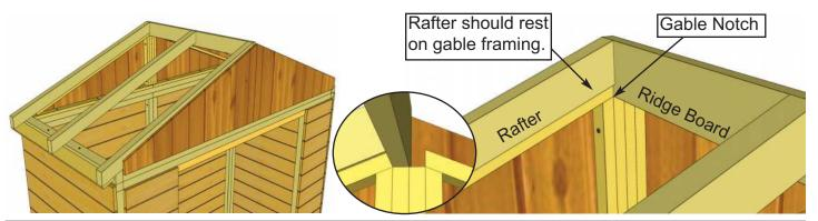
**29.** Slide Rafter section up on Gable framing until bottom of Ridge Board slips into Gable notch.
