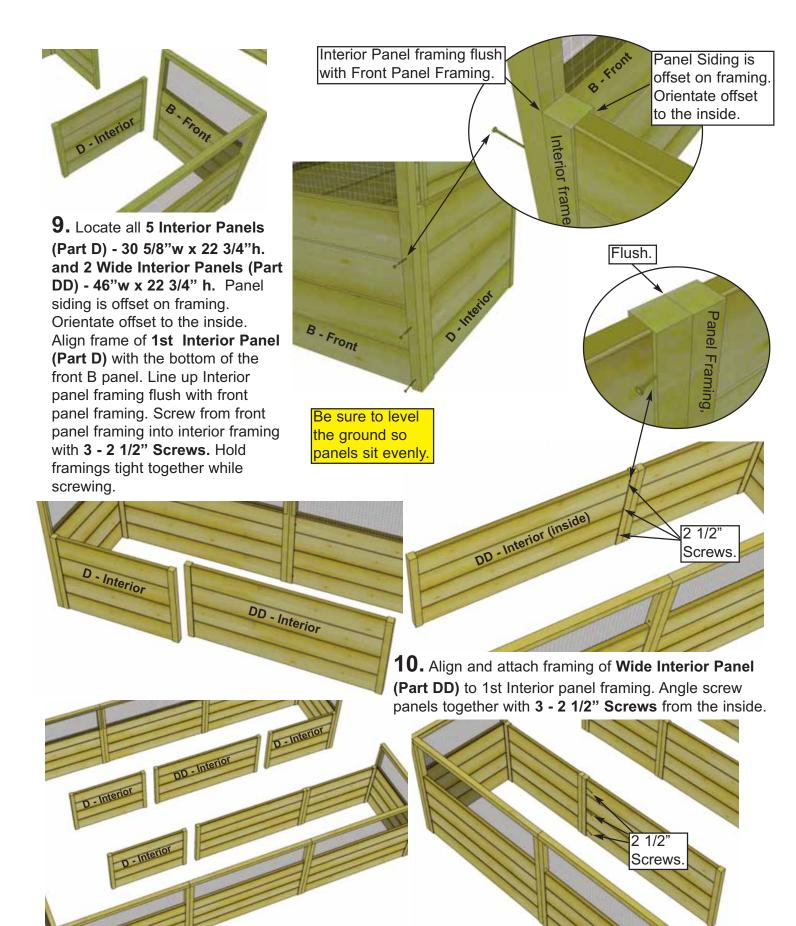
11. Align and attach framing of 3 - Interior Panels (Part D) and 1 - Wide Interior Panel (Part DD) as per Steps 9 & 10. Angle screw panels together with 3 - 2 1/2" Screws from the inside.
