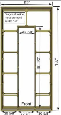
1. Orientate Panels as illustrated (screens positioned to the inside).
