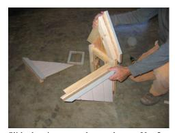
Slide the pieces together as shown. Use 2 1/2" screws to fasten together.
