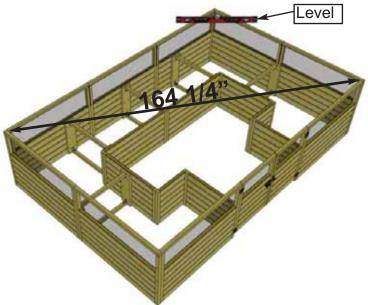
**1.** Prior to installing your Deer Fence Option Kit, confirm your 12x8 Raised Bed is level and square. Measure diagonally inside corner to corner (approximately 164 1/4") in both directions. Adjust as required. Use a level to determine if the tops of the bed frames are sloped and adjust if necessary.
