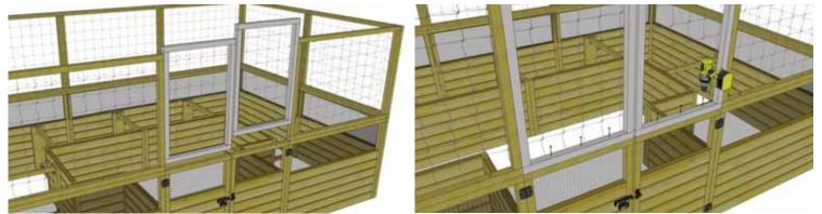
**5.** Locate both **Deer Fence Door Panels (2) - 22 3/4**" wide x 33 1/2" high. Position and install both Door Panels, screwing only from bottom frame into top of raised bed door frame with 3 - 2 1/2" screws per panel as shown above.
