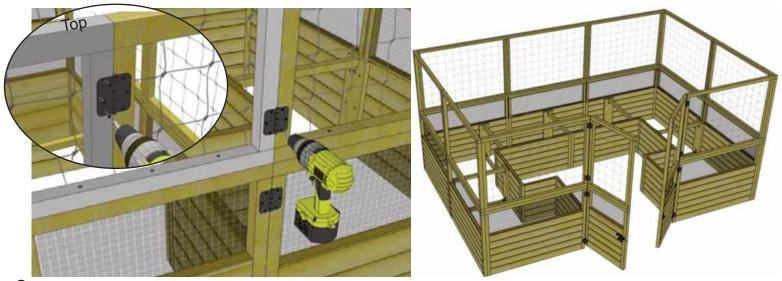
**6.** Locate all four **Black Plastic Hinges (3)** and attach to deer fence frame with **6 - 3/4**" **black screws per hinge** as shown above. Use 1/8" drill bit to pilot hole shallow holes before attaching to avoid splitting deer fence framing. Open and close door to check door aligned correctly. Adjust as required.
