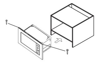
Put the microwave oven into the cabinet and keep the microwave oven in a horizontal direction and keep the edge distance of two side as same. Then fix the bolt (component 1) on the top of microwave oven and beat it into the cabinet.
