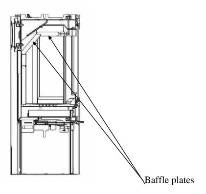
Each smoke baffle plate is to be removed separately. Both smoke baffle plates are removed by lifting up at one side after which they may come clear at the other side and be taken down into the combustion chamber and out of the door. Similarly, they are put in place by leading them up slanting-wise at one side, and then at the other side, and they are then put into place in the middle.
