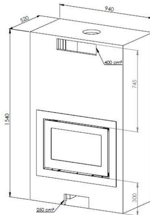
**Insulating material:** Useable are all AGI Q 132 registered insulating material. All measurements are intended as minimum distances.
