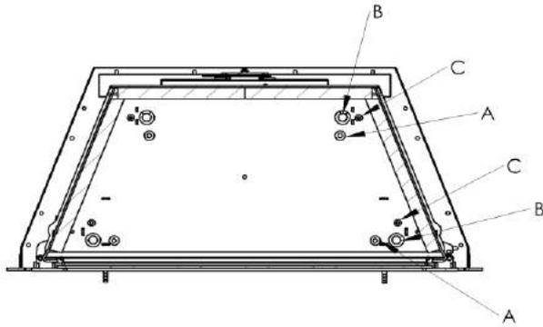
A: Holes used for fastening the insert to the base.
