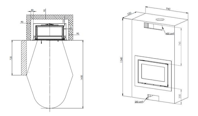
**Insulating material:** Useable are all AGI Q 132 registered insulating material. All measurements are intended as minimum distances.
