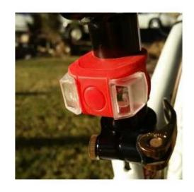
To change the taillight batteries: Pull the red silicone rubber from off the back. There will be a white plastic round cover in the back of the light. Remove that cover and there will be 2-CR2032 batteries under the cap. Replace those with 2 new CR2032 batteries positive side up. Carefully put everything back in place the way you took it apart.
